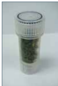
0.5 g of cannabis (hemp) before and after being ground in the GenoLyte configured for 7 mL tubes with one 1/4-inch stainless steel bead. Sample was ground for 30 seconds at the 3000 rpm setting.
