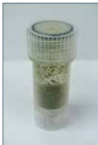
0.5 g of cannabis (hemp) before and after being ground in the GenoLyte configured for 7 mL tubes with one 1/4-inch stainless steel bead. Sample was ground for 30 seconds at the 3000 rpm setting.
