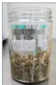
30 g sample of cannabis trimmings ground for two minutes at 1500 rpm using eight 11 mm stainless steel balls.
