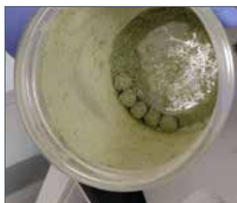
10 g sample of cannabis buds/flower ground for one minute at 1500 rpm using five 11 mm stainless steel balls.
