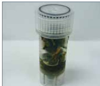
0.5 g of cannabis (hemp) before and after being ground in the GenoLyte configured for 7 mL tubes with one 1/4-inch stainless steel bead and 3 mL of EtOH. Sample was ground for 30 seconds at the 3000 rpm setting.
