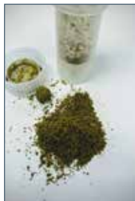
0.5 g of cannabis (hemp) before and after being ground in the GenoLyte configured for 7 mL tubes with one 1/4-inch stainless steel bead. Sample was ground for 30 seconds at the 3000 rpm setting.
