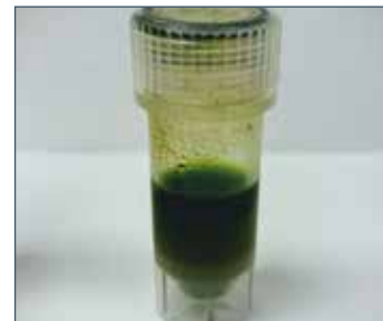
0.5 g of cannabis (hemp) before and after being ground in the GenoLyte configured for 7 mL tubes with one 1/4-inch stainless steel bead and 3 mL of EtOH. Sample was ground for 30 seconds at the 3000 rpm setting.
