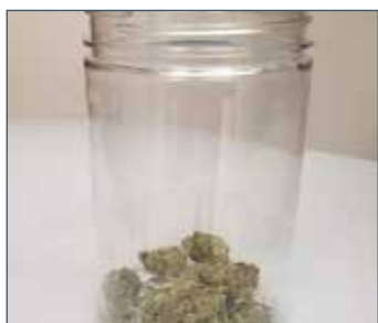
10 g sample of cannabis buds/flower ground for one minute at 1500 rpm using five 11 mm stainless steel balls.
