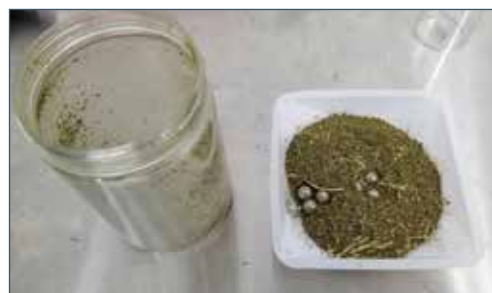
30 g sample of cannabis trimmings ground for two minutes at 1500 rpm using eight 11 mm stainless steel balls.
