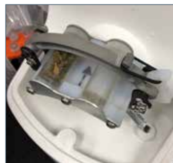
GenoLyte configured for 2 x 7 mL tubes loaded with 0.5 g of cannabis (hemp).
